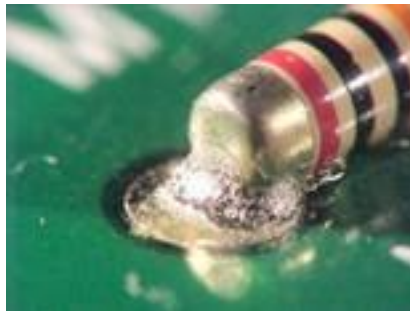
Poor Wetting Characteristics
